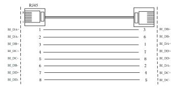
MDI/MDI-X auto connection makes switch easy to use for customers without considering the type of network cable.
